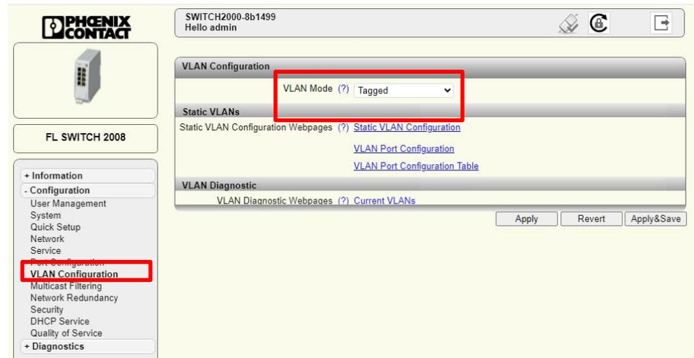
The screenshot displays the Phoenix Contact web interface for a switch (SWITCH2000-8b1499). The main content area is titled "VLAN Configuration" and includes a "VLAN Mode" dropdown menu set to "Tagged". Below this, there are sections for "Static VLANs" and "VLAN Diagnostic". The left sidebar shows a navigation menu with "VLAN Configuration" highlighted. The bottom right of the interface has "Apply", "Revert", and "Apply&Save" buttons.
